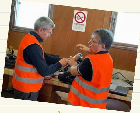
Setting the "thermal bath" (steel cylinders surrounding the OCR housings): this allows to quantify the environmental temperature "perceived" by the radiometer.
