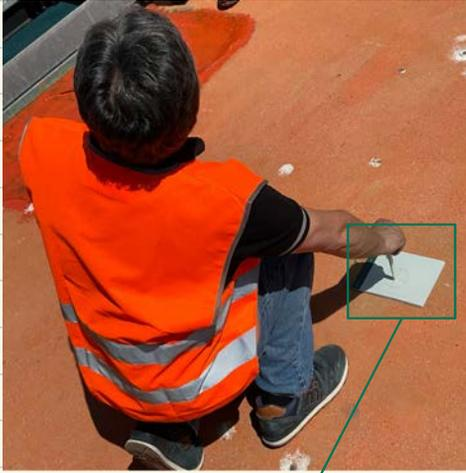
Biv-seppe explains how to azimuthally orientate the rotating stage using the spike shadow.
