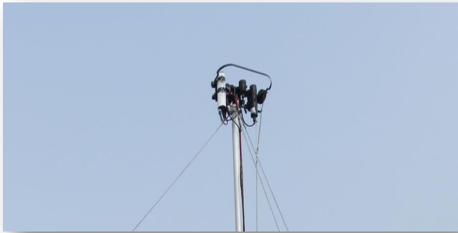
Figure 12. Set of E_s sensors deployed on a pneumatic mast equipped with a rotating shadow band attachment. The band, while moving above the sensors, obstructs the direct sun irradiance E_D(\lambda) and allows for an estimate of the diffuse component E_i(\lambda) of the total downward irradiance E_s(\lambda) .
