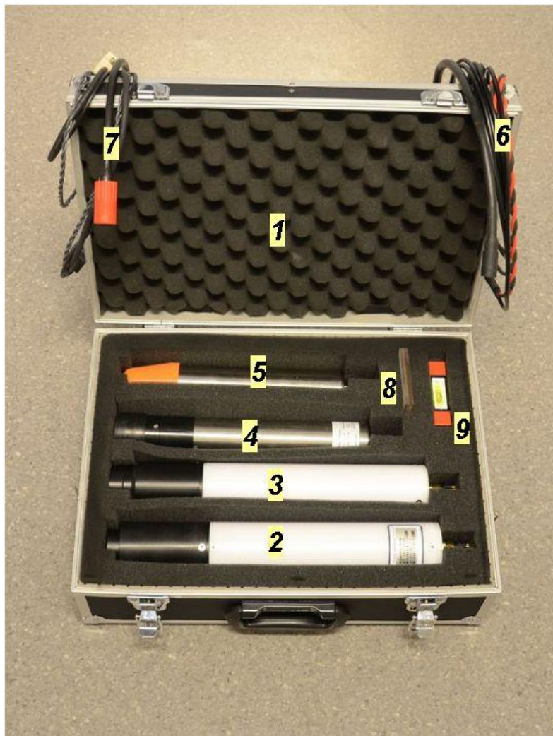
Figure 4-1. Selected radiometer models: 1 - the case, 2 - Seabird's HyperOCR radiance sensor, 3 - HyperOCR irradiance sensor, 4 - TriOS RAMSES radiance sensor, 5 - RAMSES irradiance sensor, 6 - HyperOCR connection harness, 7 - RAMSES connection harness, 8 - alignment jig, 9 - bubble level.
