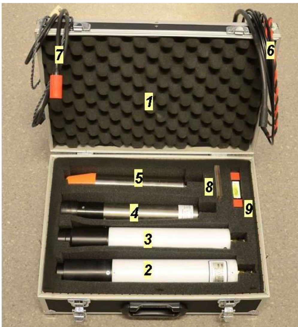
Figure 4-1. Example of radiometers characterised in the project: 1 - the case, 2 – Seabird’s HyperOCR radiance sensor, 3 - HyperOCR irradiance sensor, 4 - TriOS RAMSES radiance sensor, 5 - RAMSES irradiance sensor, 6 - HyperOCR connection harness, 7 - RAMSES connection harness, 8 - alignment jig, 9 - bubble level.
