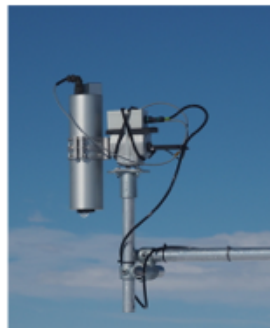
HYPSTAR® system [https://hypstar.eu/] 380-1700nm, 3-10nm FWHM
