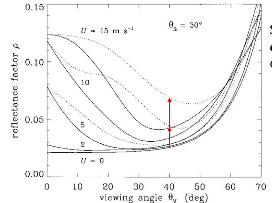
Solid lines are  $\varphi_s$  for  $135^\circ$ , dashed for  $90^\circ$ .
