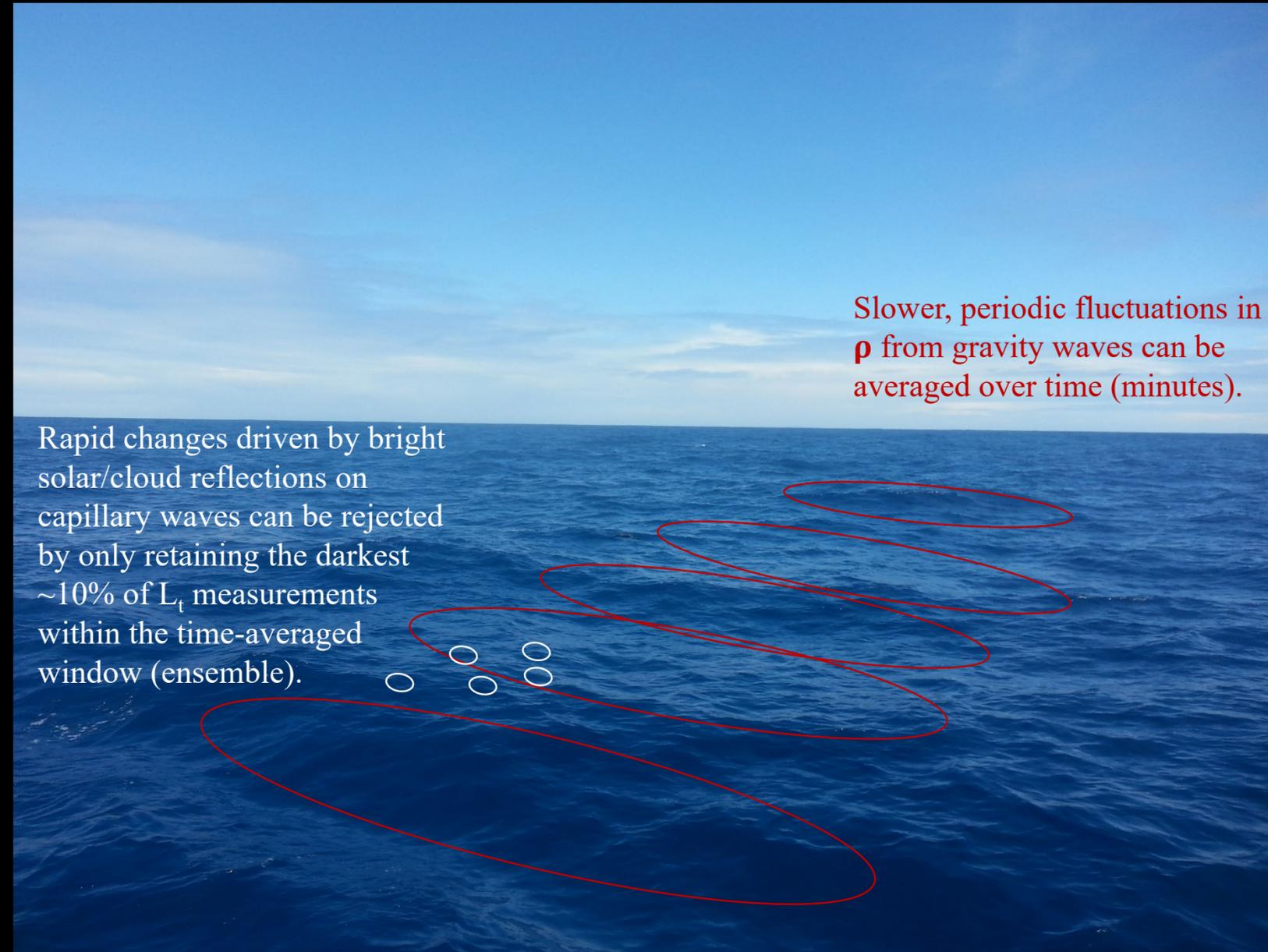
Slower, periodic fluctuations in  $\rho$  from gravity waves can be averaged over time (minutes).
