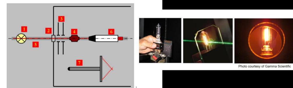
Figure 1. Pilot's (UT) irradiance calibration setup. 1 - FEL lamp; 2 - shutter; 3 - baffles; 4 - alignment laser; 5 - optical rail; 6 - radiometer; 7 - contactless distance probe.
