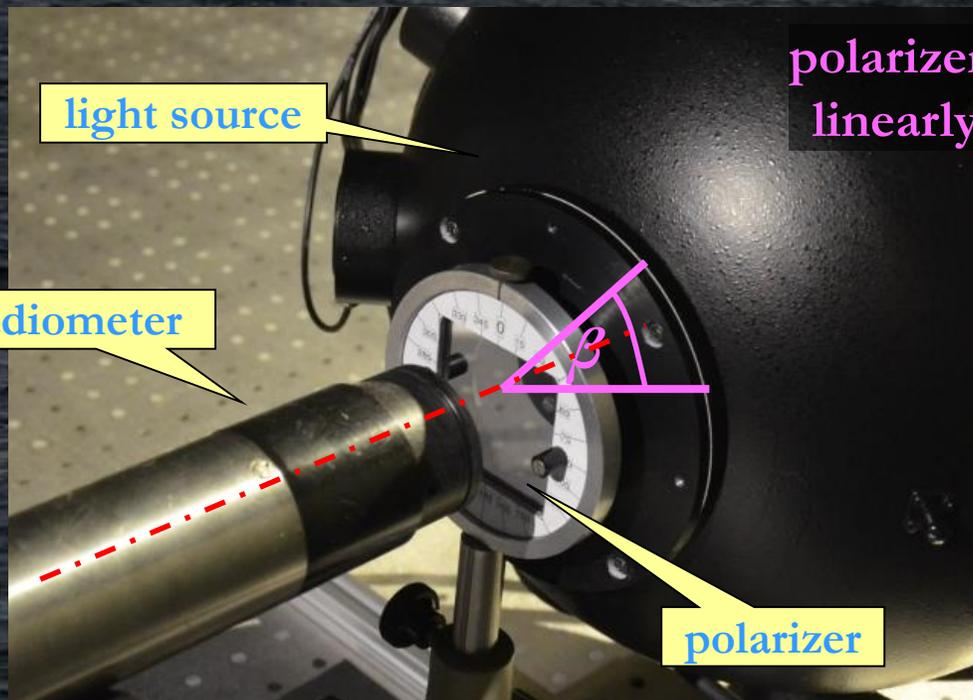
polarizer provides nearly linearly polarized light
