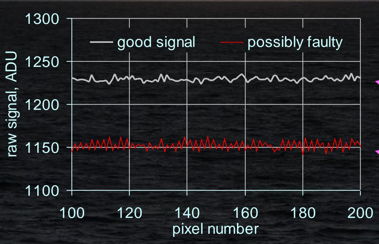
Dark signal can be sometimes used to detect hardware problems. No special equipment needed. Immunity to the electromagnetic interferences can be examined.
