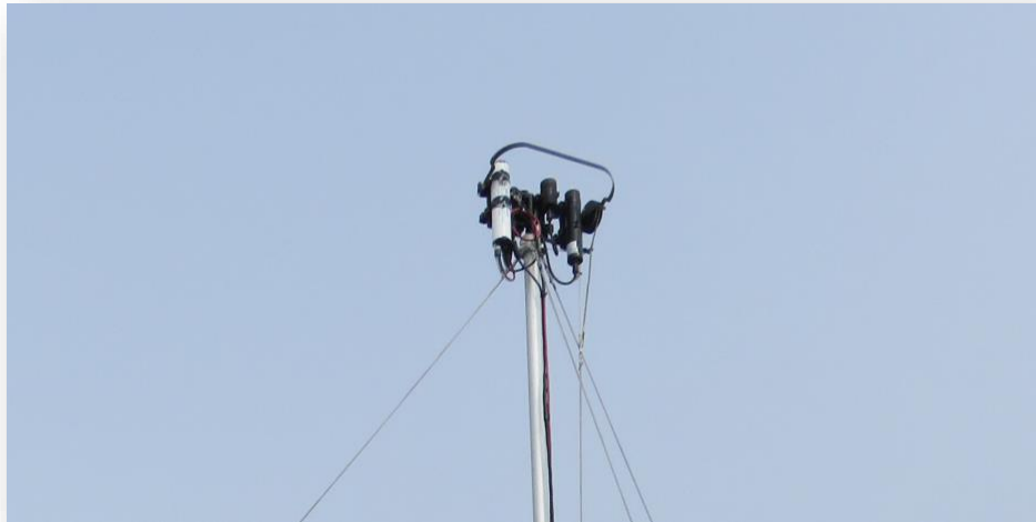
Figure 12. Set of E_s sensors deployed on a pneumatic mast equipped with a rotating shadow band attachment. The band, while moving above the sensors, obstructs the direct sun irradiance E_D(\lambda) and allows for an estimate of the diffuse component E_i(\lambda) of the total downward irradiance E_s(\lambda) .
