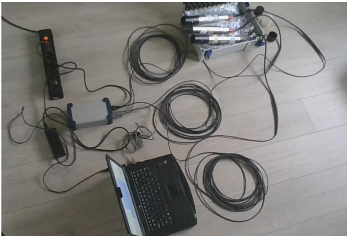
Figure 3 Radiometer measurement system consisting of (from left to right): Multi-socket power board, IPS104 radiometer power supply and data interface box, acquisition PC, RS232/USB adapter grey cable, 3*50m SUBCON/M8F RAMSES cables, box with one irradiance and two radiance TRIOS/RAMSES sensors and dummy connectors and lens caps. No external GPS is shown here since the PC internal GPS is used.
