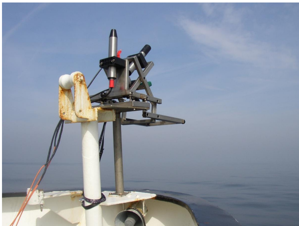
Figure 5 3-sensor abovewater radiometer system mounted at prow of ship on a steel frame with levelling screws. Reproduced from [6].
