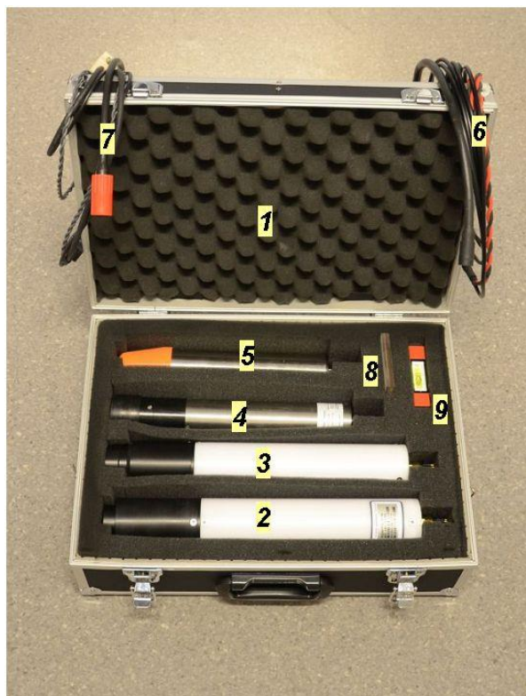
Figure 3-1. The radiometers in the focus of the document. 1 - the case, 2 - Sea-Bird's HyperOCR radiance sensor, 3 - HyperOCR irradiance sensor, 4 - TriOS RAMSES radiance sensor, 5 - RAMSES irradiance sensor, 6 - HyperOCR connection harness, 7 - RAMSES connection harness, 8 - alignment jig, 9 - bubble level.
