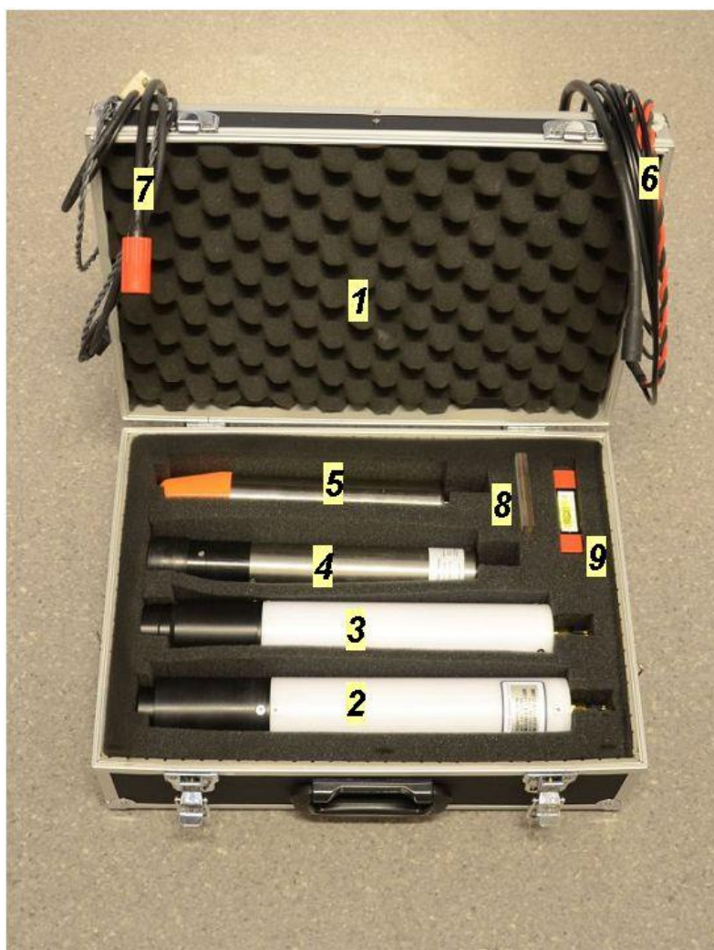
Figure 2-1. Selected radiometer models: 1 - the case, 2 - Seabird's HyperOCR radiance sensor, 3 - HyperOCR irradiance sensor, 4 - TriOS RAMSES radiance sensor, 5 - RAMSES irradiance sensor, 6 - HyperOCR connection harness, 7 - RAMSES connection harness, 8 - alignment jig, 9 - bubble level.
