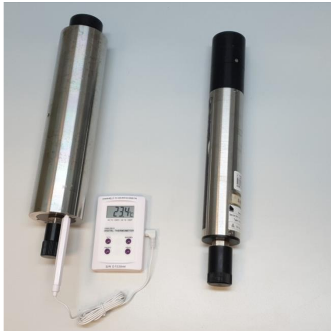
Figure 14. RAMSES sensor equipped with an external steel sleeve allowing to measure the ambient temperature in the proximity of the sensor case (left side), paralleled to the regular sensor (right side).
