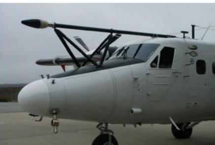
**Twin Otter has a complement of aerosol and cloud in situ probes**
