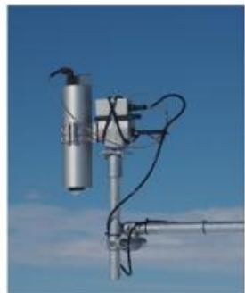
HYPSTAR® system [https://hypstar.eu/] 380-1700nm, 3-10nm FWHM
